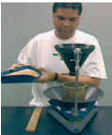
Fig. 15: Conducting a measurement of test weight (courtesy of USDA-GIPSA)
