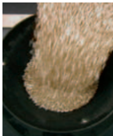
Fig. 15: Conducting a measurement of test weight (courtesy of USDA-GIPSA)
