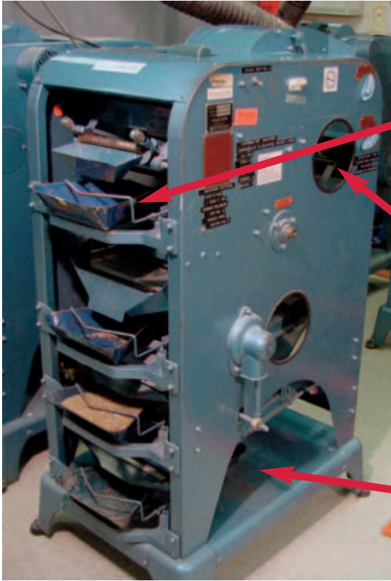
Fig. 14: Carter dockage tester (images courtesy of USDA-GIPSA)
