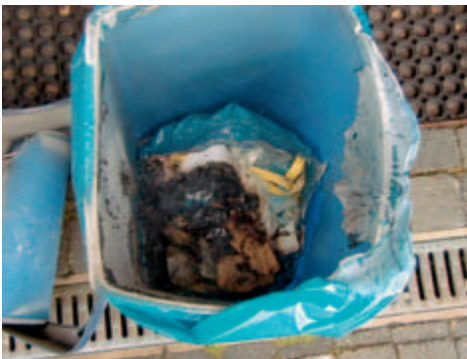
Fig. 112: Laboratory waste bin that caught fire because of mixed residues of potassium bromate and ascorbic acid
