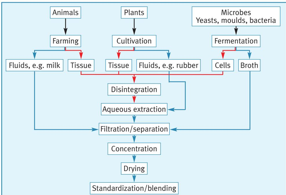
Fig. 116: Diagram showing the principle of enzyme production
