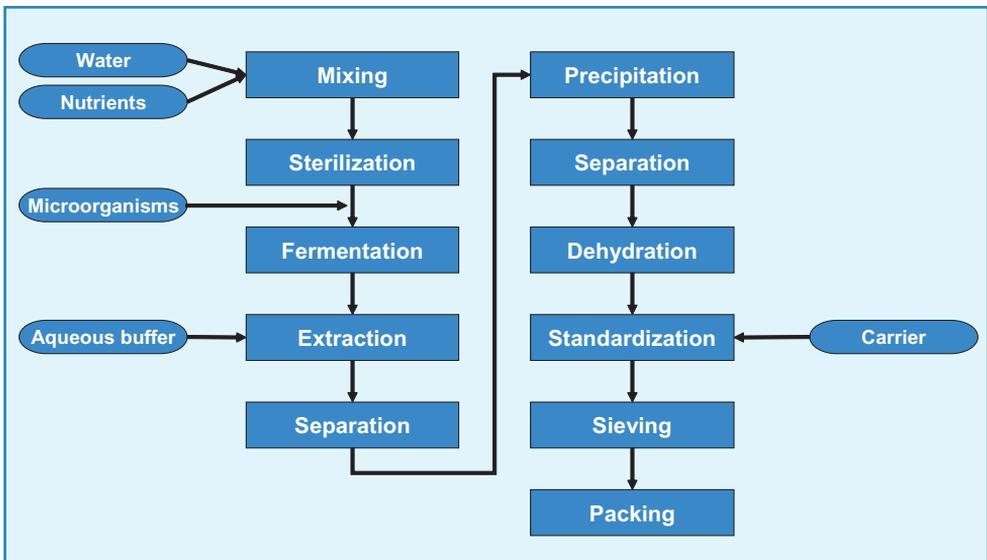
Fig. 118: Flow diagram of microbial enzyme production
