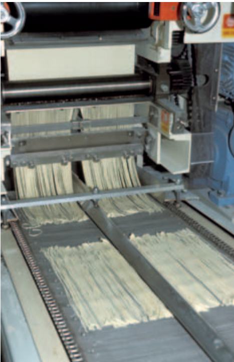
Fig. 214: Noodle (ramen) cutting machine
