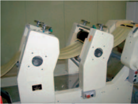
Fig. 213: Reduction rollers in a ramen line (source: H. Moegenburg, Muehlenchemie Asia Pte. Ltd.)
