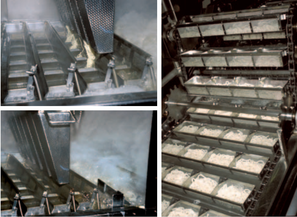
Fig. 215: Continuous cooking of udon noodles
