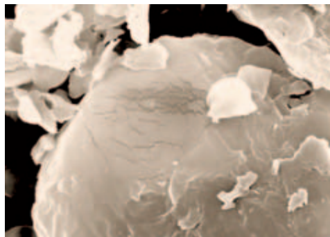
Fig. 240: SEM of a starch granule in attrition-treated flour
