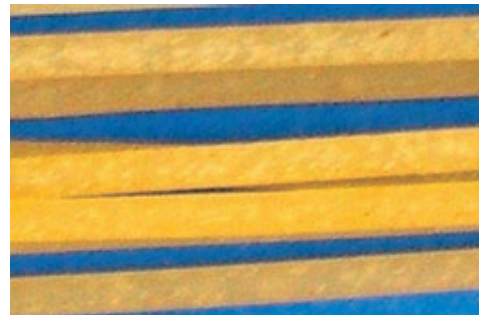
Fig. 218: Blisters in soft-wheat spaghetti caused by an inadequate vacuum during mixing.
