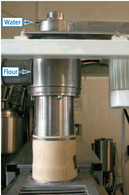
Fig. 252: Wetting unit (output approx. 1 t/h of dry substance)
